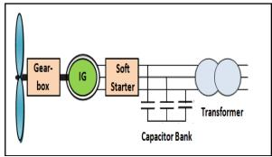
Fig. 2 Schematic diagram of Constant-speed WT
