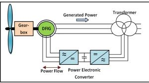
Fig. 3. Schematic diagram of DFIG based WT [36]
